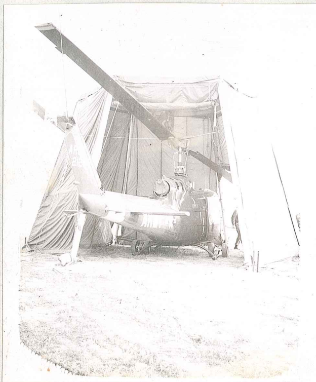
Lightweight maintenance shelter tested by the 227th.
