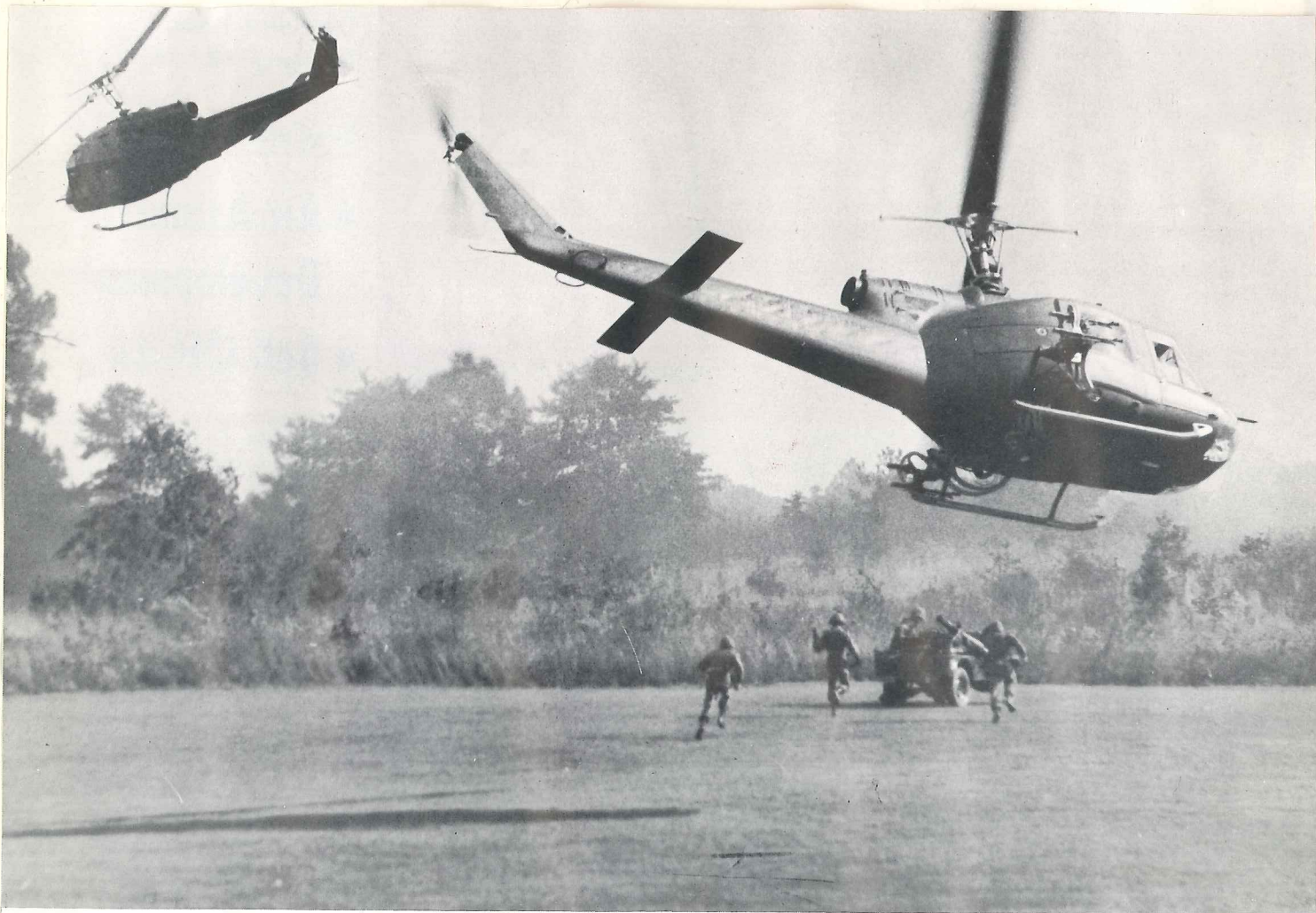
UH-1Bs LEAVE CLEARING after dropping weapons jeep and crew. Armed UH-1B mounts machine guns.
